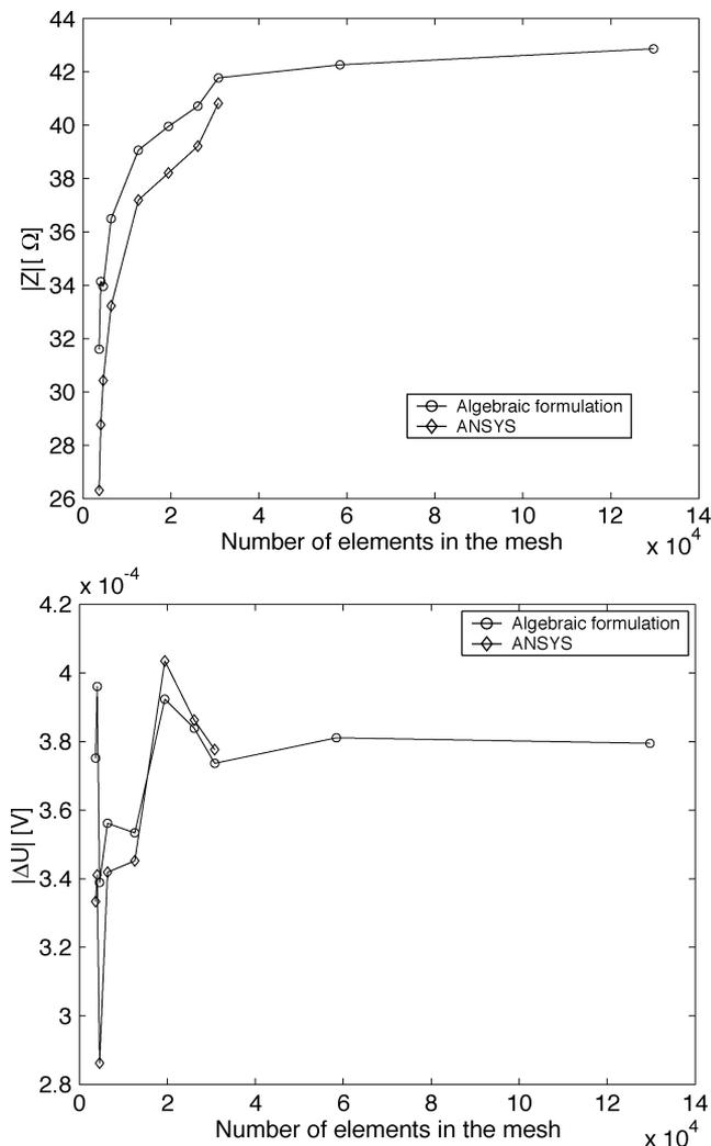
Fig. 4. Convergence of  $|Z_d|$  (on the top) and of  $|\Delta U|$  (on the bottom) values versus the number of tetrahedra.
