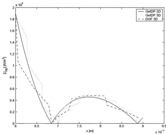
Fig. 7. Amplitude of the real part vector of the current density complex vector in the coil is shown along line 2. The discrete approach and a 2-D and 3-D analysis of GetDP are compared.
