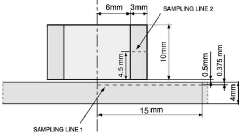
Fig. 3. Cross section of the considered geometry for the filed problem in  $D$ .
