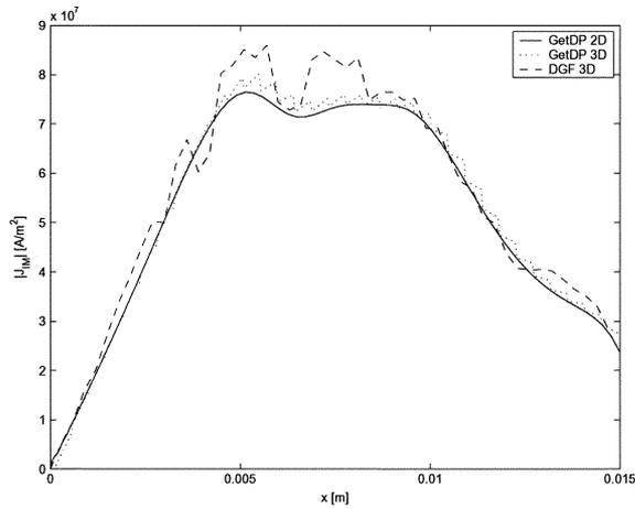
Fig. 6. Amplitude of the imaginary part vector of the current density complex vector in the plate is shown along line 1. The discrete approach and a 2-D and 3-D analysis of GetDP are compared.
