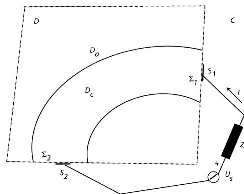
Fig. 1. Schematic view of the electromagnetic domain  $D$  containing  $D_c$  and of sources region  $D_s$ .
