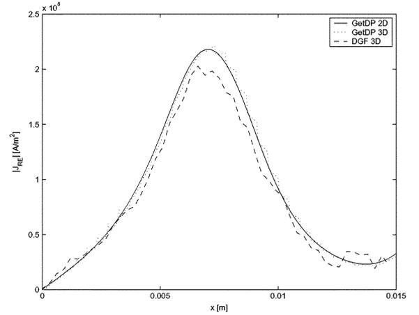
Fig. 5. Amplitude of the real part vector of the current density complex vector in the plate is shown along line 1. The discrete approach and a 2-D and 3-D analysis of GetDP are compared.
