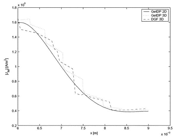
Fig. 8. Amplitude of the imaginary part vector of the current density complex vector in the coil is shown along line 2. The discrete approach and a 2-D and 3-D analysis of GetDP are compared.
