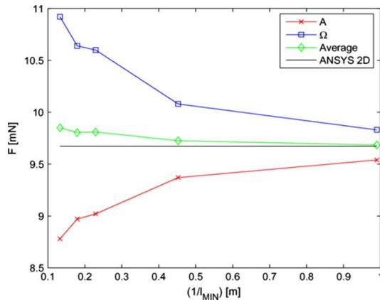
Fig. 3. Convergence of the total forces as the refinement of the mesh is increased.
