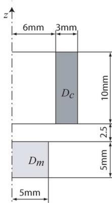
Fig. 2. Geometry of the test problem where the magnetic  $D_m$  and source  $D_c$  domains are shown.
