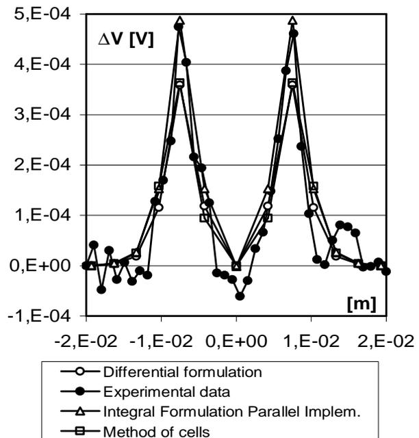
Figure 2. Comparison between numerical and experimental data for defect a) described in figure 1.
