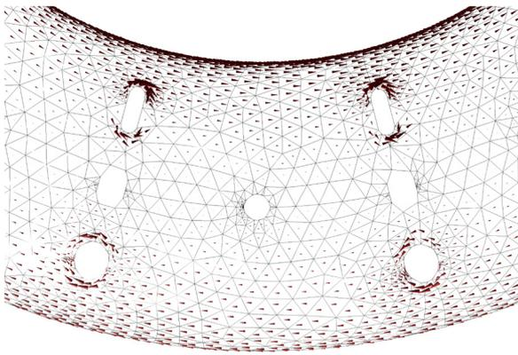
**Fig. 7.** Detail of the second reference model. The eddy currents are induced by a uniform vertical magnetic field (sinusoid at  $f=100$  Hz). Red cones: real part of the current density (a.u.), not to scale. (For interpretation of the references to color in this figure legend, the reader is referred to the web version of this article.)
