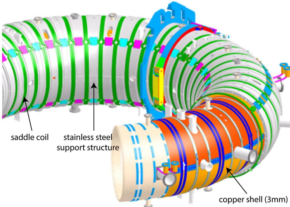
**Fig. 5.** Cutaway of the torus assembly of RFX-mod device. The main passive conducting structures (copper shell, stainless steel toroidal support structure) are shown together with a subset of the 192 ( $48 \times 4$ ) saddle coils, used for active control of MHD instabilities.
