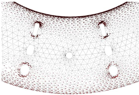
**Fig. 7.** Detail of the second reference model. The eddy currents are induced by a uniform vertical magnetic field (sinusoid at  $f=100\text{ Hz}$ ). Red cones: real part of the current density (a.u.), not to scale. (For interpretation of the references to color in this figure legend, the reader is referred to the web version of this article.)
