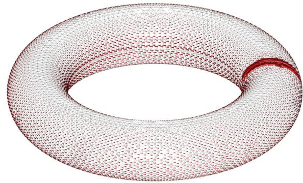
**Fig. 6.** Eddy currents induced in the first reference conducting structure by a uniform vertical magnetic field (sinusoid at  $f = 100$  Hz). Red cones: real part of the current density (a.u.), not to scale. (For interpretation of the references to color in this figure legend, the reader is referred to the web version of this article.)
