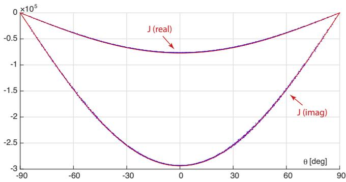
**Fig. 3.** Current density (real, imaginary) induced on the hollow sphere as a function of the azimuthal angle  $\theta$ : comparison between the proposed approach (dots) and the reference solution (solid lines).
