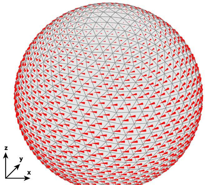
**Fig. 2.** Eddy currents induced by a vertical magnetic field on a hollow sphere discretized with 1888 triangles, 2832 edges, 946 nodes. Red cones: real part of the current density (a.u.), not to scale. (For interpretation of the references to color in this figure legend, the reader is referred to the web version of this article.)
