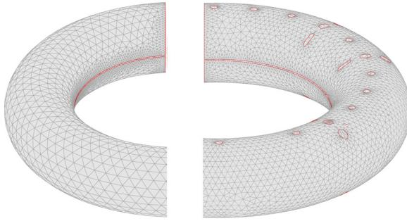
**Fig. 4.** (a) A torus with two gaps, discretized with 10,641 triangles, 16366 edges, 5726 nodes. Only half of the model is shown. (b) A torus with two gaps and several holes, discretized with 21,097 triangles, 32,776 edges, 11,606 nodes. Only half of the model is shown.
