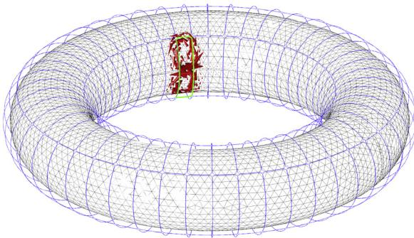
**Fig. 8.** Eddy currents induced in the first reference structure by a time varying magnetic field. The source is an inner coil (green) out of the 192 ( $48 \times 4$ ) saddle coils of the feedback system used to control MHD instabilities in RFX-mod. Red cones: real part of the current density (a.u.), not to scale. (For interpretation of the references to color in this figure legend, the reader is referred to the web version of this article.)
