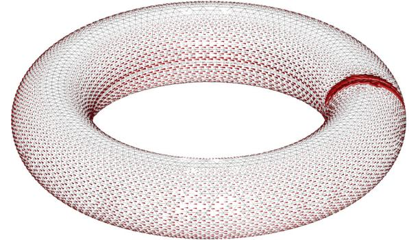
**Fig. 6.** Eddy currents induced in the first reference conducting structure by a uniform vertical magnetic field (sinusoid at  $f=100\text{ Hz}$ ). Red cones: real part of the current density (a.u.), not to scale. (For interpretation of the references to color in this figure legend, the reader is referred to the web version of this article.)
