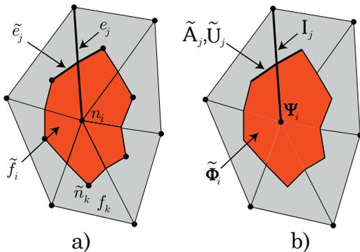
Fig. 1. (a) Geometric elements of the primal and dual complex. (b) Association of the physical variables to geometric elements of the primal and dual complex.
