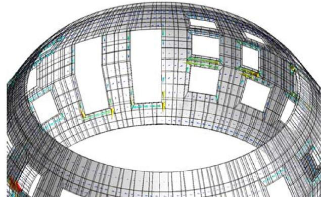
**Fig. 8.** Detail of the current density in the stabilizing plate.
