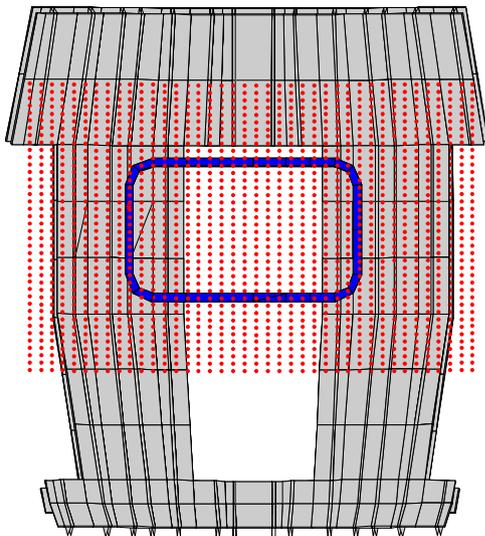
Fig. 2. A detail of the SP implemented in the symmetric geometry for CAFE (stiffening ribs are included), together with a RWM coil and the grid of points used for field calculations.
