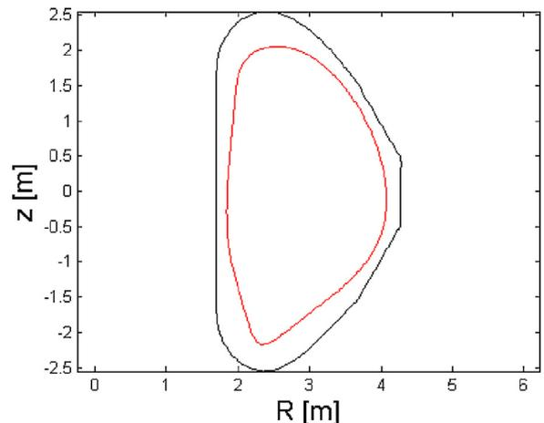
Fig. 5. Plasma boundary and poloidal trace of the 2D continuous wall located at the stabilizing plate.
