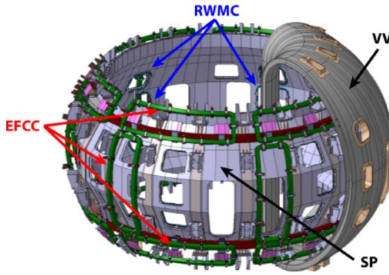
**Fig. 1.** JT-60SA. The control coils (RWMC, EFCC) are shown together with the stabilizing plate (SP) and the vacuum vessel (VV). [JT-60SA Research Plan, ver. 3.1].
