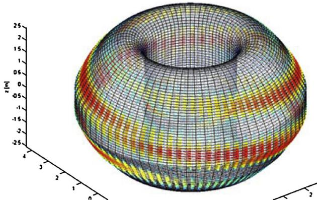
Fig. 7. 3D view of the current density pattern corresponding to the unstable eigenmode.
