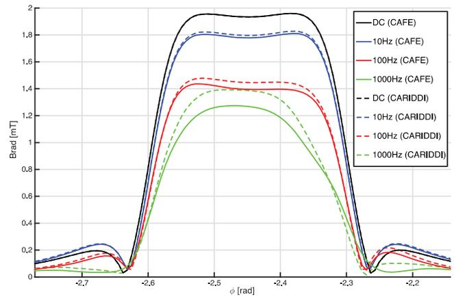
Fig. 4. Magnetic field amplitude (radial component) computed from DC to 1 kHz in a subset of the gridpoints shown in Fig. 2 (horizontal line at z = 0 m,  $\Delta\phi = \pm 10^\circ$ ).
