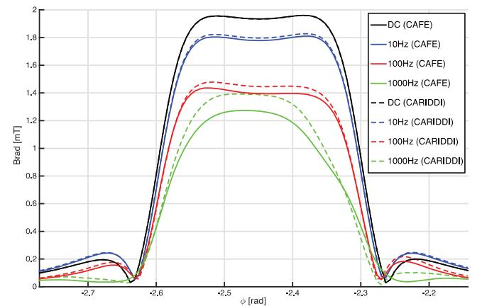
**Fig. 4.** Magnetic field amplitude (radial component) computed from DC to 1 kHz in a subset of the gridpoints shown in Fig. 2 (horizontal line at  $z=0$  m,  $\Delta\phi=\pm 10^\circ$ ).
