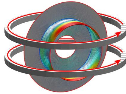
Fig. 9. 3-D (non-axisymmetric) current density pattern induced by two circular loops (ac current,  $f = 50$  Hz) series connected. Colored cones: real part of the current density. The hotter the color, the higher the current density.
