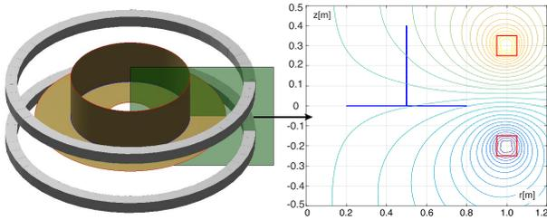
Fig. 6. Left: 3-D problem with cylindrical symmetry. A conducting structure (uniform resistivity  $\rho = 0.1 \mu\Omega$  and thickness  $\delta = 1$  mm) placed in the region between a pair of coils. Right: 2-D view. The magnetic field produced by the coils (ac current,  $f = 50$  Hz, anti-series connected) is also shown.
