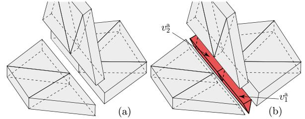
Fig. 3. (a) Primal complex of each manifold part is constructed independently. Again, manifold parts are drawn exploded for clarity. (b) Manifold parts are stitched back together by adding prismatic volumes as  $v_1^a$  and  $v_2^a$ .
