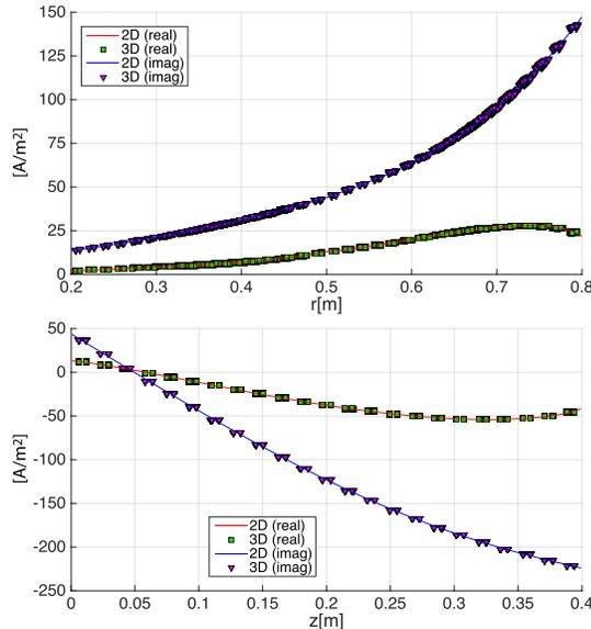
Fig. 7. 3-D solution versus 2-D: real and imaginary parts of the current density ( $J_\phi$  component) induced in the drilled disk (top— $z = 0$  m and  $r = 0.2 \div 0.8$  m) and in the cylinder (bottom— $r = 0.5$  m and  $z = 0 \div 0.4$  m).
