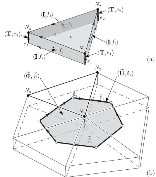
Fig. 1. Association of physical variables to geometric elements of (a) primal and (b) dual complexes.
