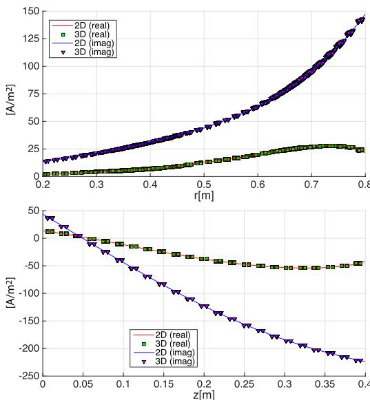
Fig. 7. 3-D solution versus 2-D: real and imaginary parts of the current density ( $J_\phi$  component) induced in the drilled disk (top— $z = 0$  m and  $r = 0.2 \div 0.8$  m) and in the cylinder (bottom— $r = 0.5$  m and  $z = 0 \div 0.4$  m).
