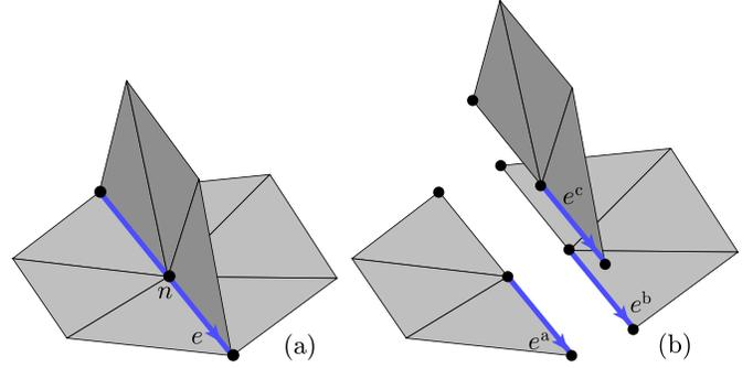
Fig. 2. (a) Non-manifold discrete surface  $\mathcal{S}$ . Non-manifold edges, as  $e$ , and non-manifold nodes are marked. (b)  $\mathcal{S}$  is cut into a minimal number of manifold parts. The manifold parts are drawn exploded for clarity, but the coordinates of the triplicated nodes are inherited from the original node.
