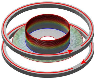
Fig. 8. 3-D solution of the problem shown in Fig. 6. The conducting structure is discretized with 17144 triangles, 26187 edges, and 9043 nodes (157 non-manifold). Colored cones: real part of the induced current density. The hotter the color, the higher the current density.
