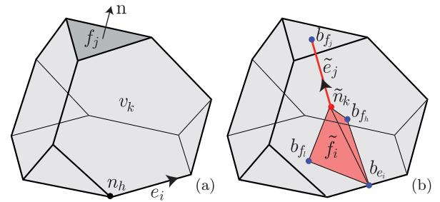
Fig. 1. (a) Edge  $e_i$  and a face  $f_j$  of a polyhedron  $v_k$  in  $\mathcal{K}$ . (b) Dual face  $\tilde{f}_i = D(e_i)$  dual to edge  $e_i$  and dual edge  $\tilde{e}_j = D(f_j)$  dual to face  $f_j$ .
