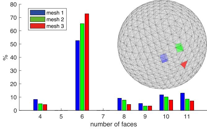
Fig. 3. Percentage of different kinds of polyhedra used in sphere's meshes 1 (coarse), 2 (intermediate), and 3 (fine). Inset: mesh 1: a tetrahedron (red), a hexahedron (blue), and a polyhedron with 11 faces (green) are shown.
