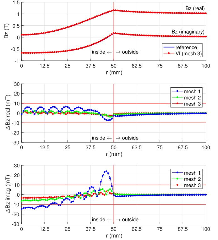
Fig. 4. Top: comparison of computed (VI) versus reference (analytical) solution in terms of  $B_z$  (real and imaginary components) along a radial path ( $y = 0, z = 0, x \in [0, 100]$ ). Middle and bottom:  $\Delta B_z$  real and imaginary components.
