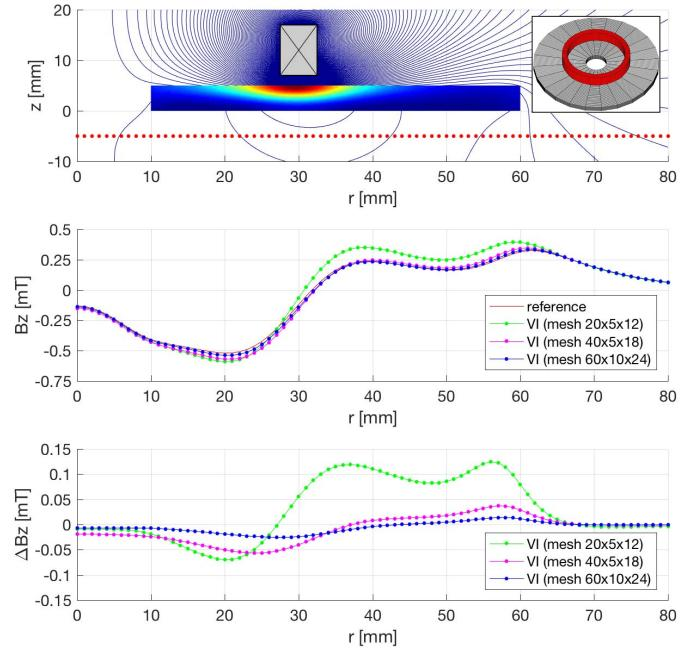
Fig. 5. Top: 2-D axisymmetric reference configuration (stranded coil, 1000 ampere-turns,  $f = 1$  kHz, above a thick copper disk with one hole). Inset: 3-D mesh ( $60 \times 10 \times 24$ ). Middle: VI versus reference.  $B_z$  (real component) along the radial path in the top figure (red dots) for three meshes. Bottom:  $\Delta B_z = B_z^{VI} - B_z^{ref}$  (real component).
