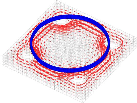
Fig. 6. Conducting domain is discretized in 1656 polyhedra, 5736 faces, 6567 faces, and 2484 nodes. The field source is an axisymmetric coil (blue) fed by an ac current at  $f = 50$  Hz. Red cones: real part of  $\mathbf{J}$ , not to scale.
