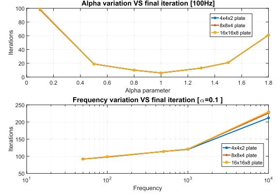
Fig. 3. Top: required iterations with relaxation parameter  $\alpha$  and mesh grain variation. Bottom: required iterations trend with frequency and mesh grain variation.
