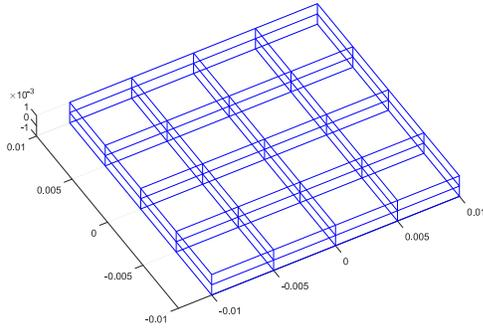
Fig. 2. Slab with coarsest discretization.
