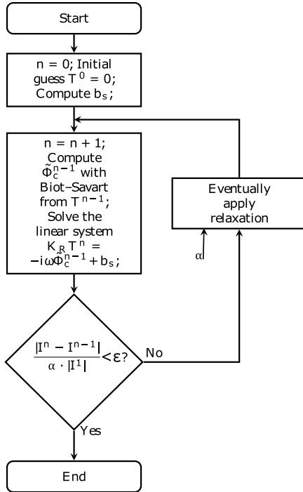
Fig. 1. Iterative solution of an eddy current problem.
