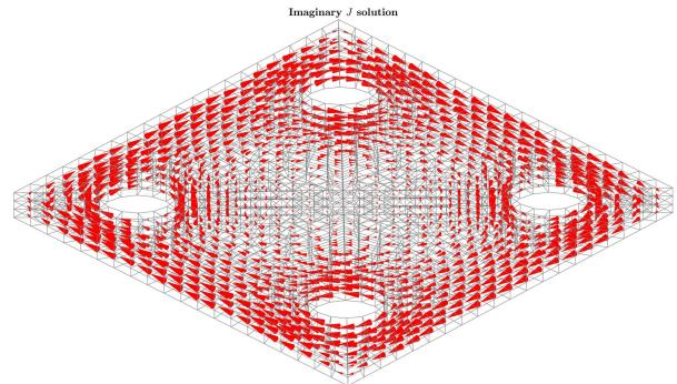
Fig. 7. Imaginary part of the eddy current induced in the conducting structure.
