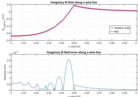
Fig. 6. Magnetic induction field due to the imaginary part of the eddy current induced in the sphere and related absolute error.
