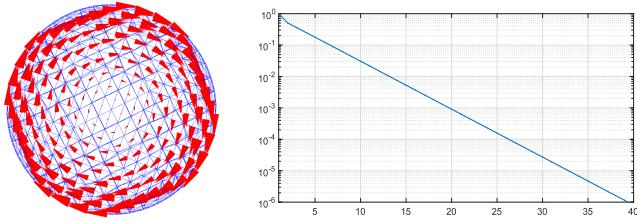
Fig. 5. Left: eddy currents induced in a solid sphere (radius  $r = 50$  mm and resistivity  $\rho = 0.1 \mu\Omega\text{m}$ ) subject to a uniform sinusoidal magnetic field ( $B = 1$  T and  $f = 50$  Hz) in the direction perpendicular to the page; red cones are the imaginary part of the current density. Right: convergence of the method. Current update is a function of the number of iterations  $n$ .
